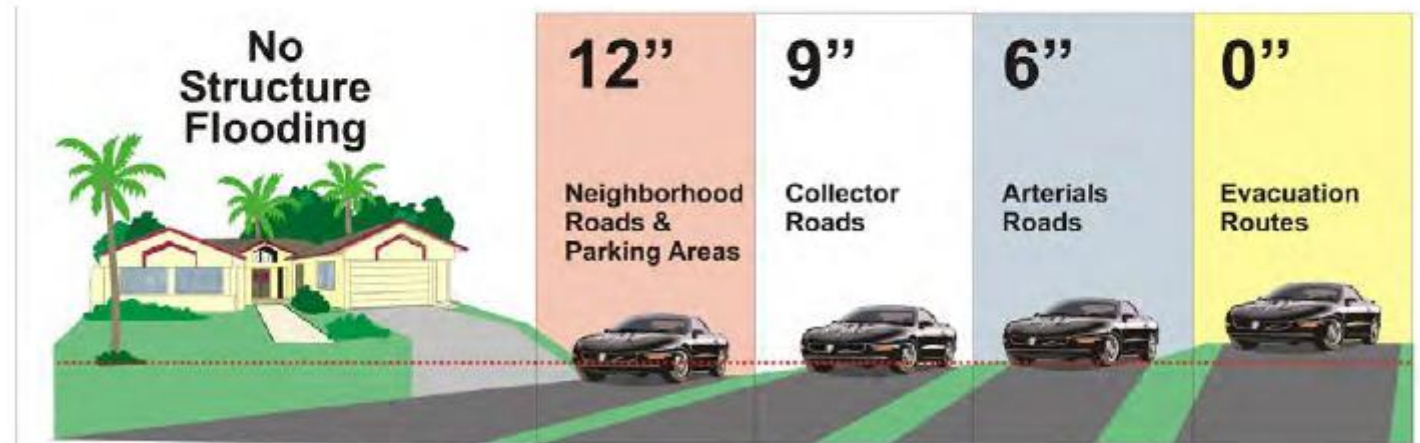
Figure 4-1 Acceptable Flooding for a 100-Year Storm
