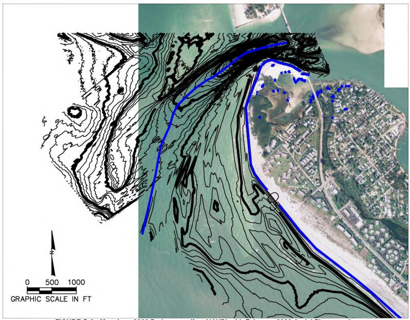
FIGURE C-8: May-June 2006 Bathymetry (feet NAVD) with February 2006 Aerial Photograph.
