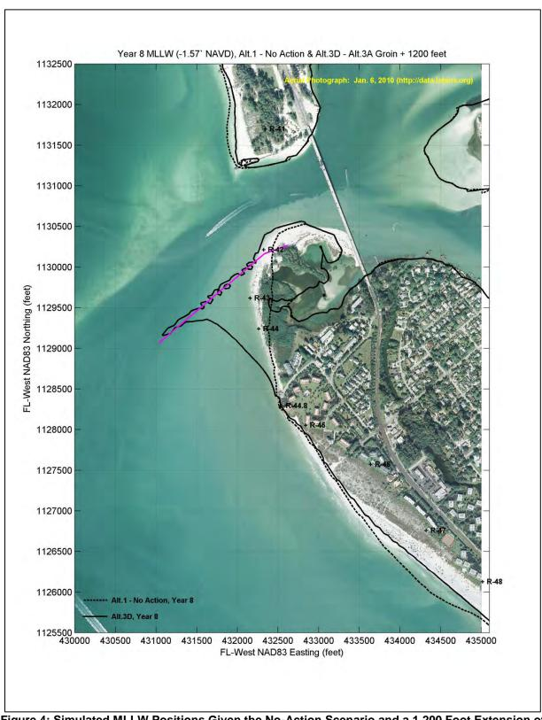
Figure 4: Simulated MLLW Positions Given the No-Action Scenario and a 1,200 Foot Extension of the Alt. 3A Groin.
