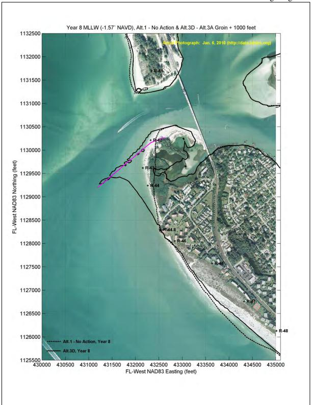
Figure 3: Simulated MLLW Positions Given the No-Action Scenario and a 1,000 Foot Extension of the Alt. 3A Groin.
