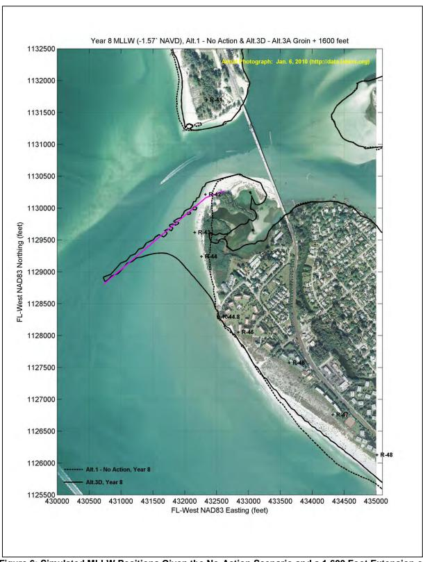
Figure 6: Simulated MLLW Positions Given the No-Action Scenario and a 1,600 Foot Extension of the Alt. 3A Groin.
