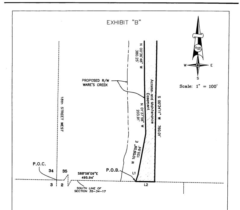
Line Length Bearing 25.77 N18'18'38"E L1 L2 68.47 N88'58'09"W
